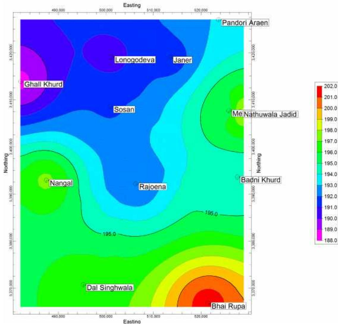
The data is validated by selecting the deepest well in each quadrant with those supported electrical logs for preparation of aquifer map and is shown below
