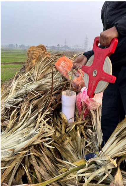
Water Level Monitoring in Bore well Rafiganj.
