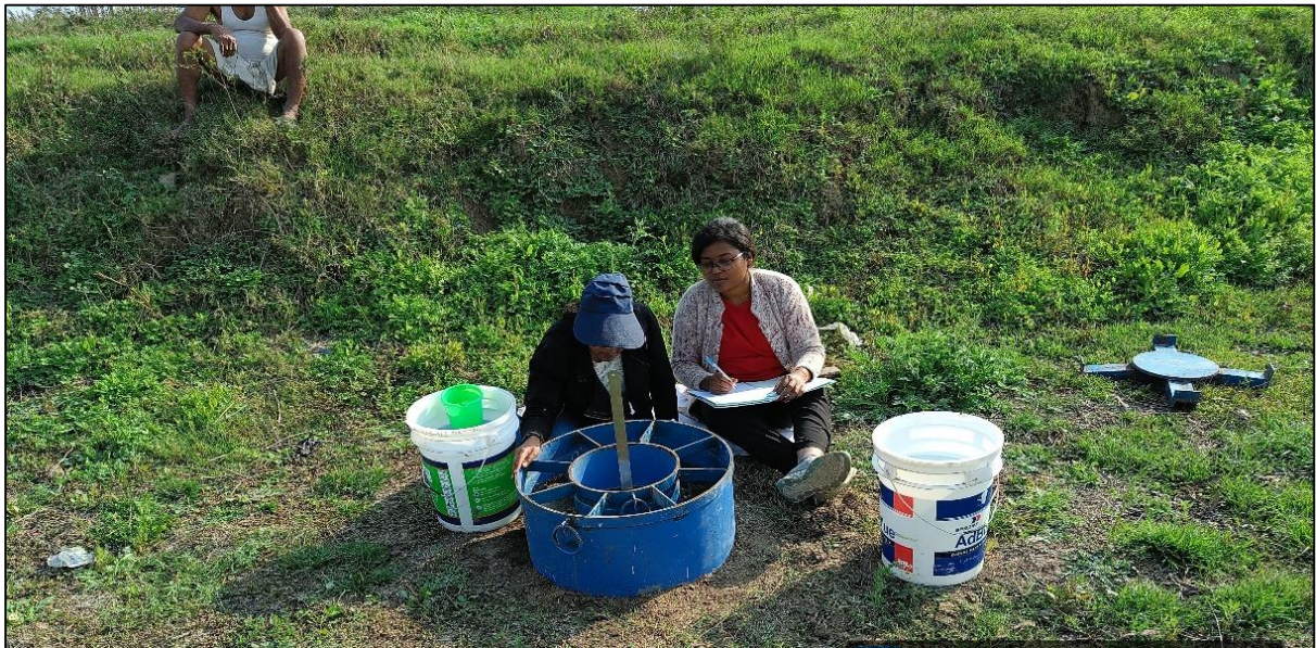
Figure 14: Field photograph of soil infiltration test using double ring infiltrometer technique.
