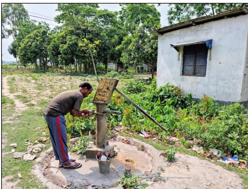
Inventory of India Mark-II tube well at Bhojo Gobindo Roy Madhyamik Shiksha Kendra, Birghai village (Raiganj block) during village level aquifer mapping survey
