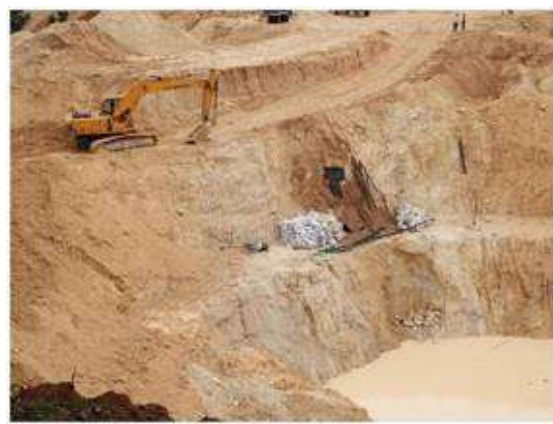
Photo 4: Deep weathering in Singhbhum Granite, observed from road cut. Its more clayey in nature
