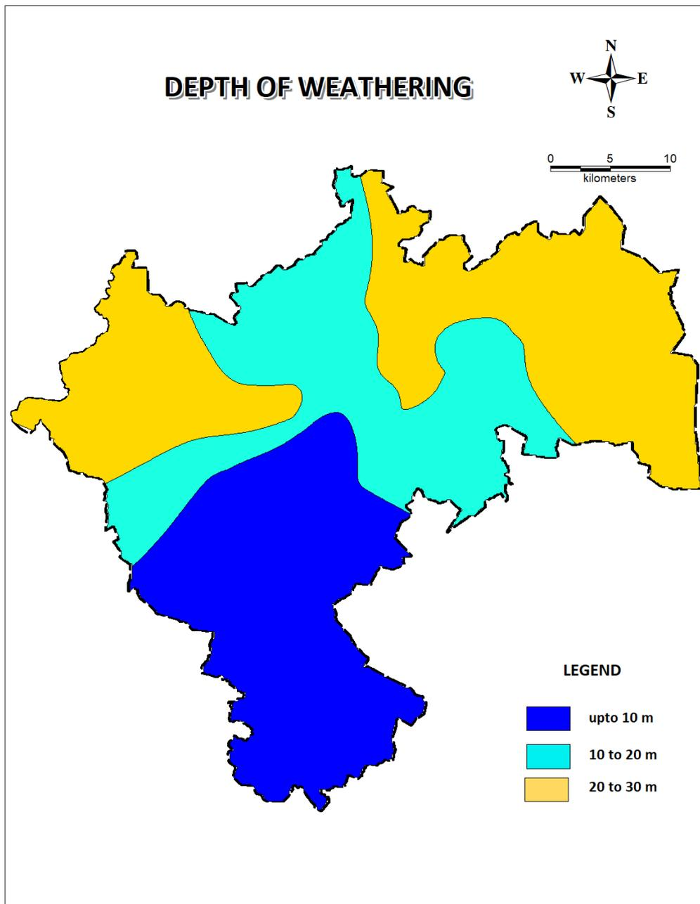
**Figure 2.2. Depth to weathering map-Hosanagara Taluka.**
