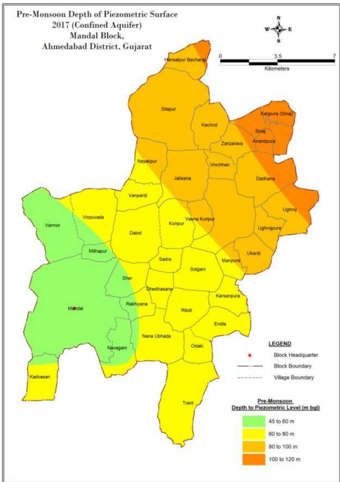
Fig.11: Pre-Monsoon Depth of Piezometric Surface- Confined Aquifer
