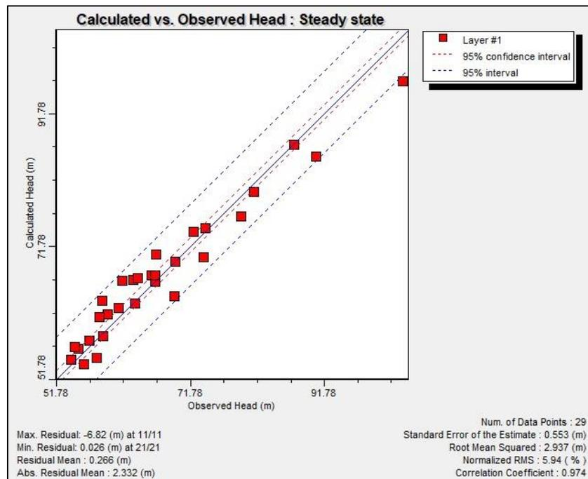
Fig 11: Head Scatter Graph for Steady State
