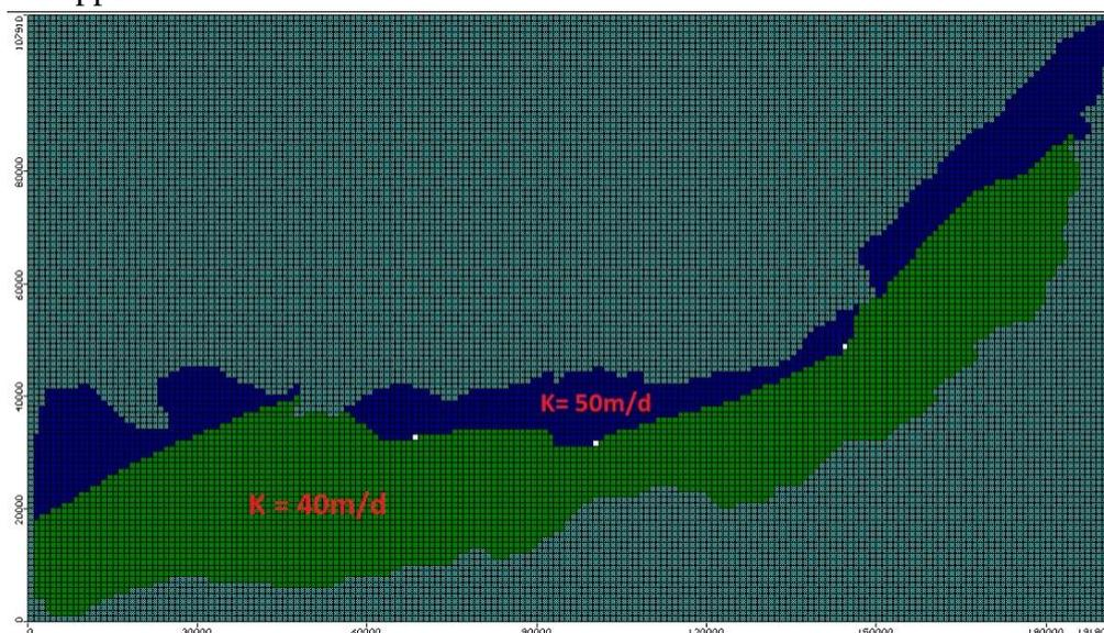
Fig 9: Horizontal Hydraulic Conductivity zones in the Area
