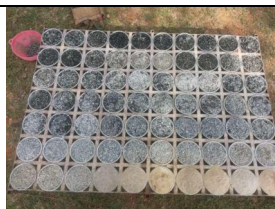
Fig. 9b: Litholog samples collected during drilling at T.B.Colony EW site
