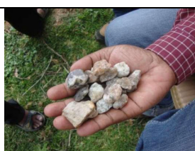
Fig. 9c: Fractured litholog sample at deeper depth (162 m bgl) collected during drilling at Sasalu site
