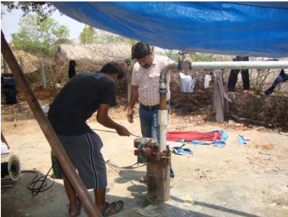
Monitoring of ground water level during pumping test at Huchanahatti EW site
