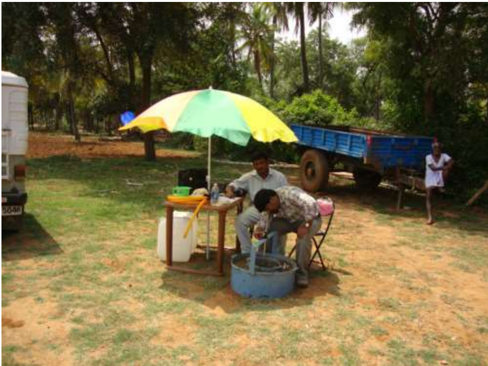
Double ring infiltration test at Rudrapura village
