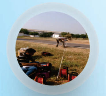
Resistivity survey for site selection at Army Station at Talbehat, Bundelkhand
