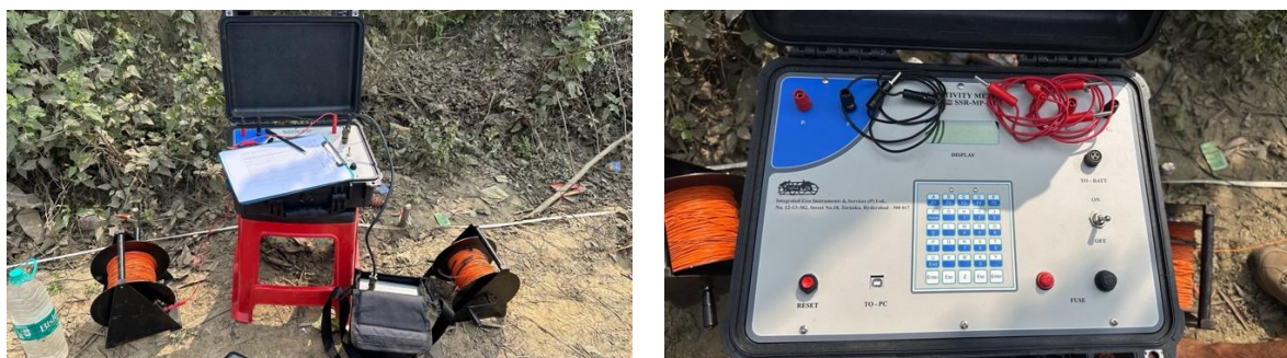
Figure 5-2: SSR MP ATS Instrument used for VES Survey in the Study Area
