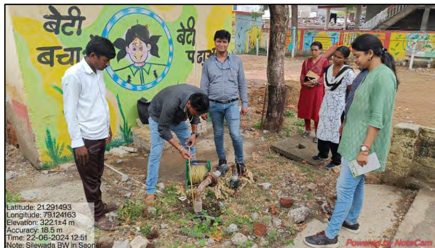
Fig. 9.4 Measurement of Bore well showing declining water level in Silewara village near mining area.
