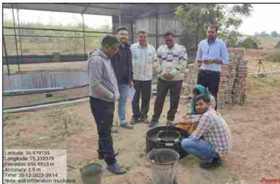
Figure-7.1: Soil Infiltration test in field.
