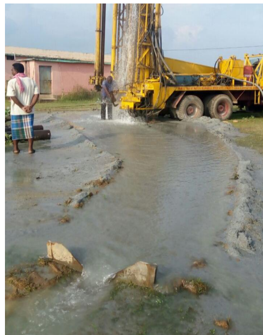
Fig 3.5-Exploratory Well drilled at Nawagaon, Block-Bagbahera, District- Mahasamund (CG), Discharge with 18 lps
