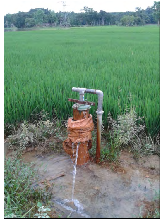
Fig 4.3: Pumping Test at Kochewahi District Durg Fig 4.4: Auto flowing Irrigation TW at Paschim Jalefa, Satchand Block, Tripura
