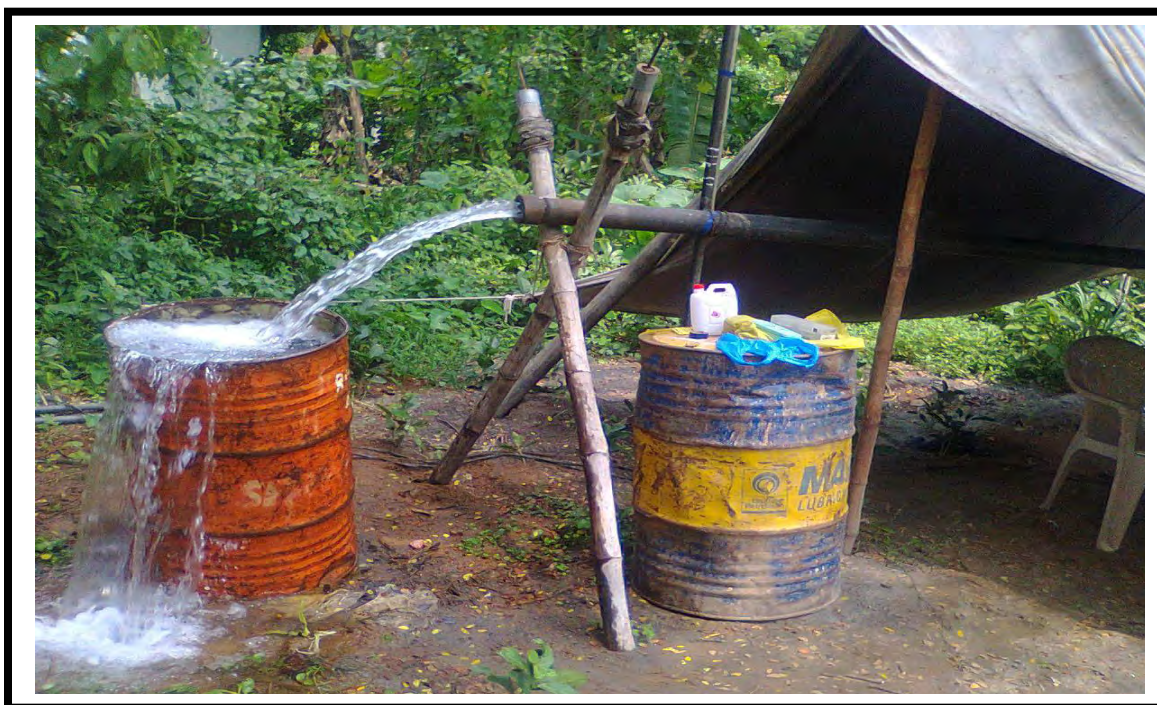
Fig 4.2 Aquifer Performance test at Exploratory well , Kothamangalam, Ernakulam district, Kerala.
