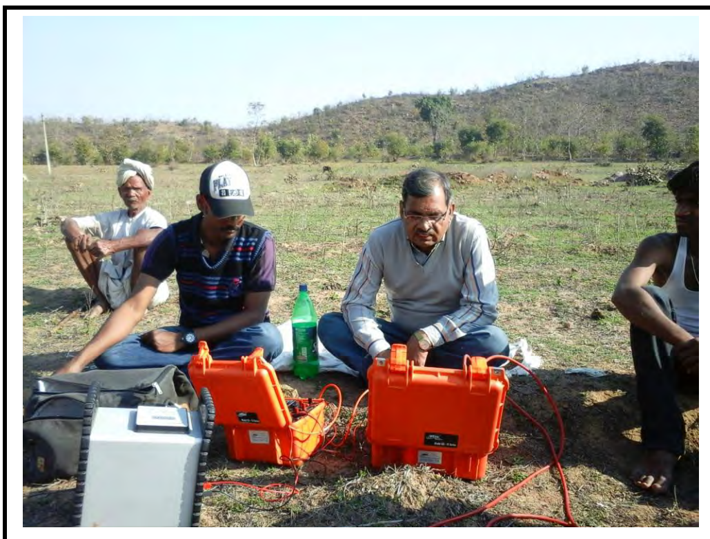
Fig. 5.1 Conducting Resistivity survey in Chhattarpur distt. (M.P.)
