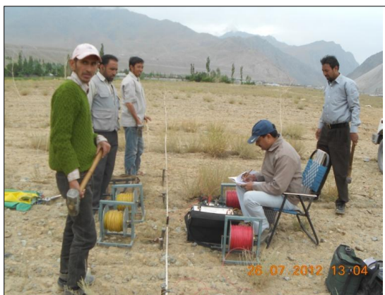
Fig 2.7 Resistivity Surveys at SKUAST, Kargil district (J&K)
