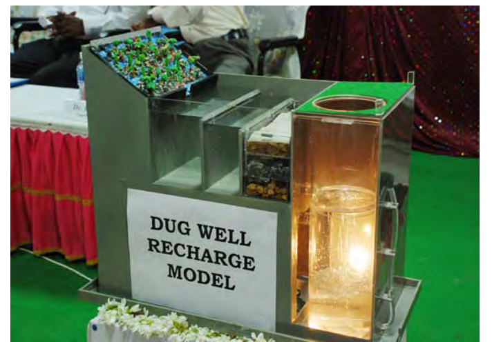
Dug Well Recharge Model
